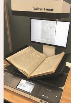
Therefore, with the board’s authorization, the BAP recently purchased an archiving machine. The BookEye 4v2 (pictured) has a scanning surface that is 17½” tall and 24” wide, and scans two pages in one pass. The laser sensor keeps the type in focus for clear copies of any document. With this kind of quality, the BAP can preserve its priceless documents for the future.
